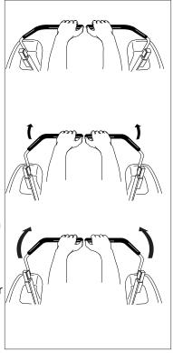
Figure 3. Move Control Levers Gradually
